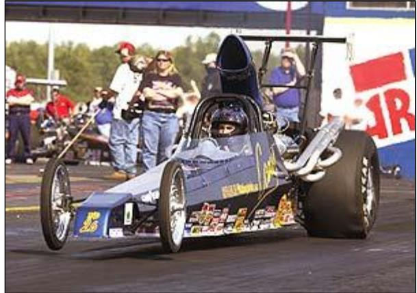
Casey's car is based on a 235-inch Spitzer chassis. Amazingly, the only change necessary for Casey's leg was to add a 2-inch block to the brake pedal.
